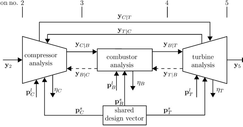
**Figure 1 Coupled core engine design problem**
